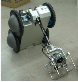
Fig. 2. Camera arm capable of lifting up the robot.
